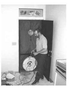
The blower door test does not measure air leakage. It is a measurement of the size of all the holes in the home. This is converted to an estimate of average annual air leakage by applying some math to the blower door test results. The final result is called ACH Natural.
