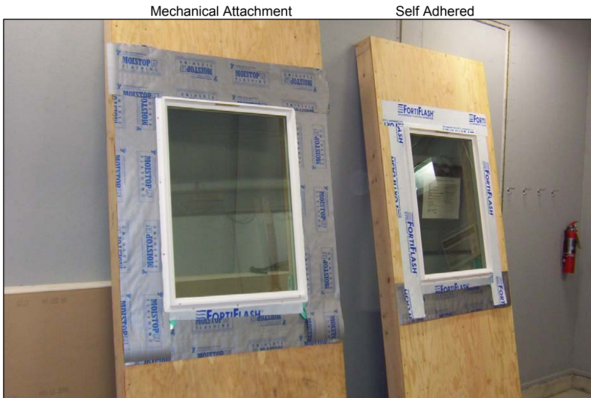
Figure 18 Window flashing detail prior to the addition of building paper
