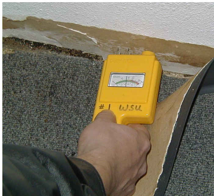
A moisture meter at work.
