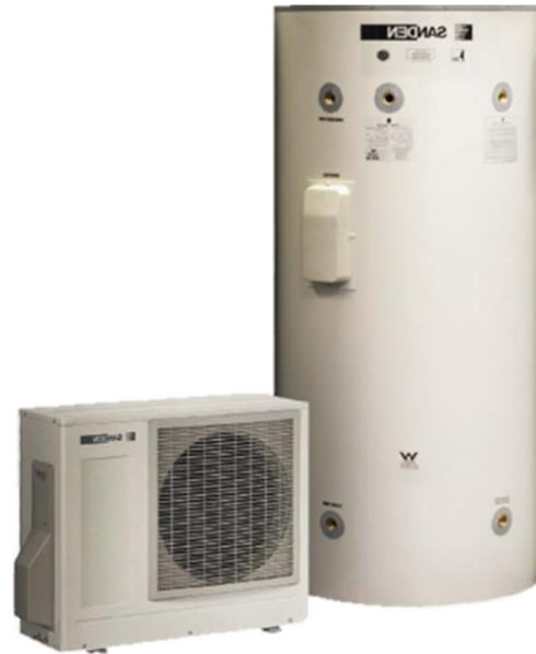
A sensor wire connects the tank temperature sensor to the control system in the outdoor unit. The controls turn the system on and off for water heating, operate the defrost cycle to prevent icing in cold weather, and circulate hot water to prevent freezing of the lines and heat exchanger during long periods of system inactivity in cold weather.
