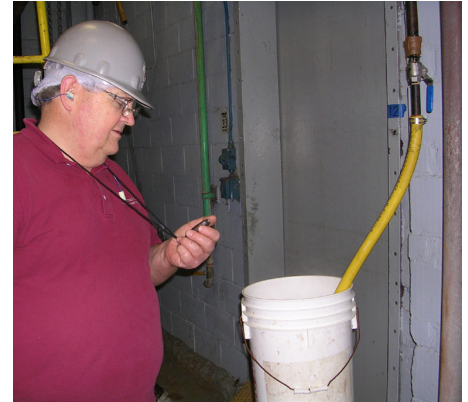
An engineer verifies water flow rate using the bucket and stop watch method.
