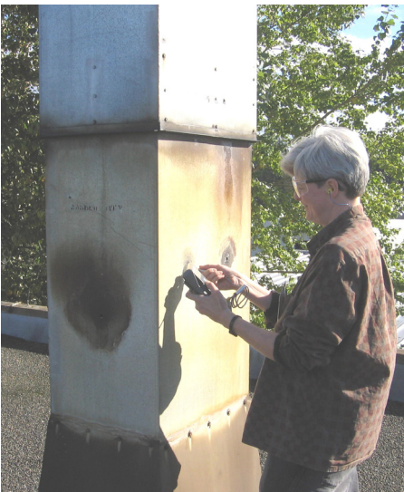
An Energy Engineer monitors the temperature and oxygen content of flue gas.
