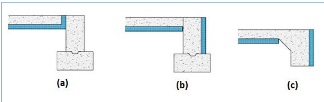
**What are prescriptive slab insulation requirements for below-grade walls and slabs?**
