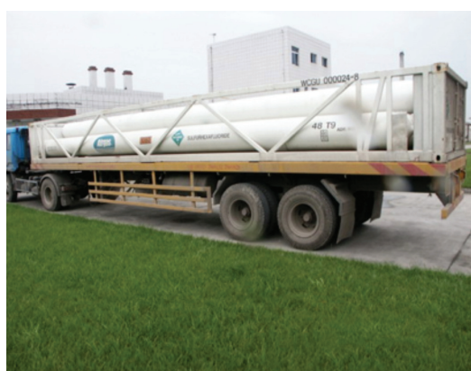
CNG tube trailer delivers gas directly to the end user.
